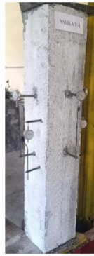
Fig 4. Installation of devices to measure the average relative deformations in the reinforcement
