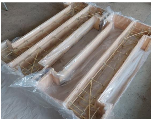
Picture 2. Preparation of reinforcement frames and placement in molds.
