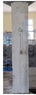
Fig 4. Installation of devices to measure the average relative deformations in the reinforcement
